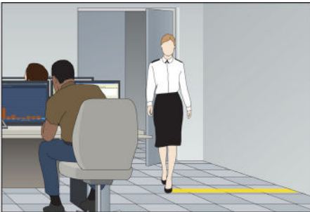
When a person walks across the floor, the friction generates minimal static, and the flooring material dissipates the charge safely to ground.
