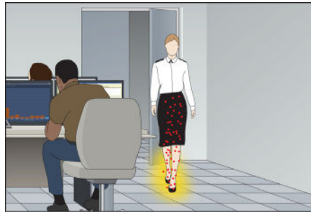
A person enters the room. Friction between the soles of her shoes and flooring material generates static. As she crosses the floor, a static charge builds on her body.
