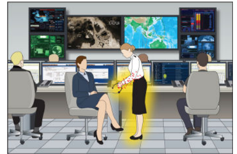
The static electricity on her body discharges to the first person or object she touches—in this case, the headset.
