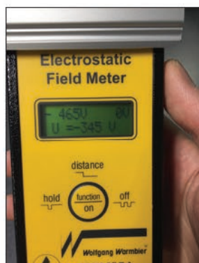
Figure 2: Body voltage measured per ANSI/ESD STM 97.2 ( V = 465 volts) test method on a person wearing two ESD heel straps while walking on a static dissipative floor measuring 5.5 \times 10^6 RTG. Note, the upper limit for V per ANSI/ESD S20.20 is 100 volts.
