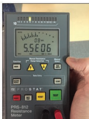
Figure 1: Actual resistance to ground (RTG = 5.5 \times 10^6 ) measurement on a static dissipative vinyl floor with a poly-urethane low maintenance coating. Note, the upper limit for RTG per ANSI/ESD S20.20 is less than 1.0 \times 10^9 .
