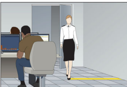
When a person walks across the floor, the friction generates minimal static, and the flooring material dissipates the charge safely to ground.
